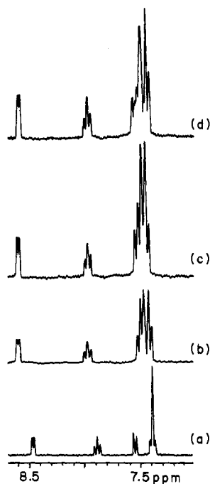
Figure 6. ^1\text{H} NMR Spectra (300 MHz, \text{D}_2\text{O} ) of (a) carbinoxamine maleate (0.025 M) with (b) \beta -cyclodextrin (0.025 M), (c) 6- \beta -CD-EN-DTPA (0.025 M), and (d) 2- \beta -CD-EN-DTPA (0.025 M).
